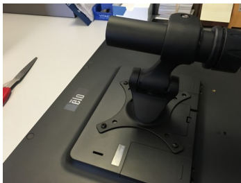
Screw back (VESA Mount) into tablet (screen) using the Phillips head screws supplied by stand manufacturer (Peerless)
