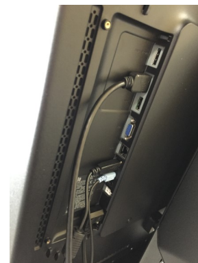
Newer ELO screen models will have their cable and power source connections vertically accessible on the back side of the screen.
