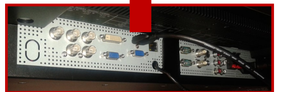
The cable and power source connections to the NEC screens are accessible underneath the screen
