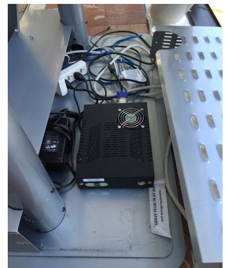
Ensure the player is free of debris so air can circulate and keep the player from overheating.
