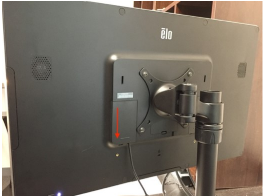
Slide off the rectangular panel on the back of the tablet
